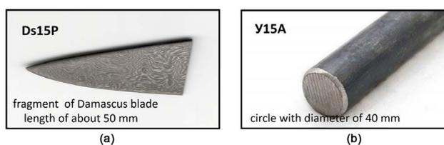
**Figure 1.** Research materials: (a) genuine Damascus steel; (b) carbon Tool steels.
