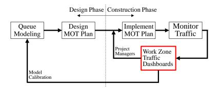
Figure 1. Work zone maintenance of traffic plan development flow chart.
