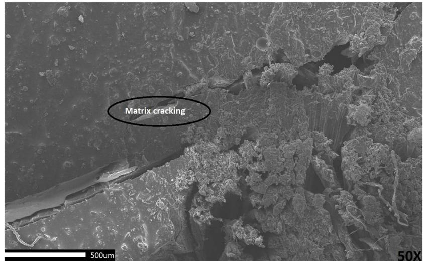
**Figure 2.** Matrix cracking of an immersed sample due to attacks by the water molecules (50× Magnification).
