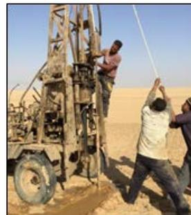
**Figure 6.** Standard penetration test (SPT) during wash mechanical drilling.
