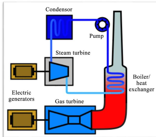
**Figure 1.** Combined Cycle Power Plant CCPP diagram [23].
