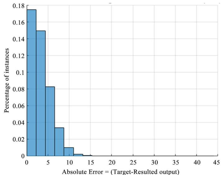
**Figure 13.** Absolute Output power (PE) Error (MW) vs. percentage of Instances (Complete dataset).
