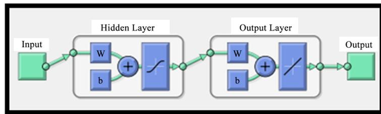
**Figure 3.** Universal approximating network (Regression Neural Network Structure [28]).
