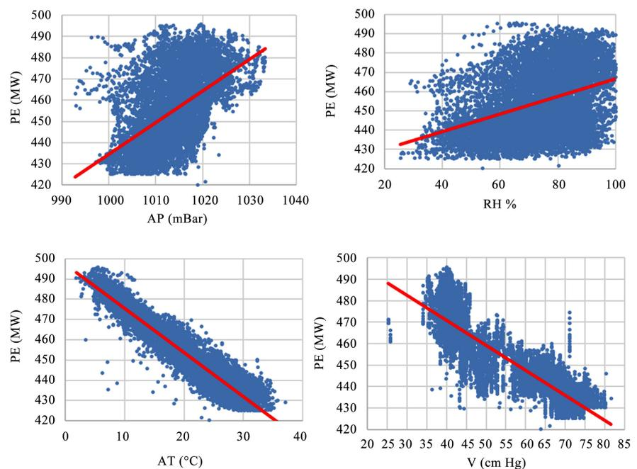
**Figure 2.** Linear Correlation between inputs and output PE.
