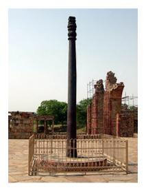
**Figure 1.** The iron pillar of Delhi, India [Chemical composition: 0.15% carbon, 0.25% phosphorus, 0.005% sulfur, 0.05% silicon, 0.02% nitrogen, 0.05% manganese, 0.03% copper, 0.05% nickel, and balance iron] [7].
