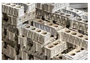
**Figure 6.** Mg alloy motorcycle engine blocks to minimize fuel consumption through weight saving [11].
