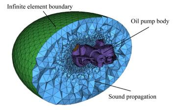
Figure 2. The established finite element model of the gear pump.
