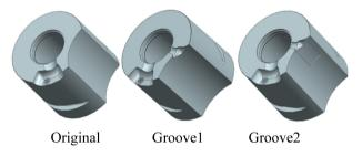
Figure 6. The shape of unloading groove.
