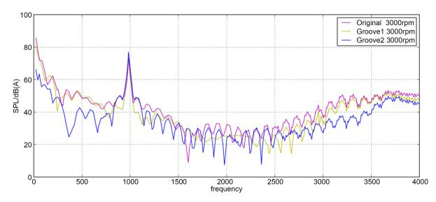
**Figure 7.** Sound pressure spectra: simulation results of original pump, unloading groove pump and unloading groove and diversion groove pump at 3000 rpm.
