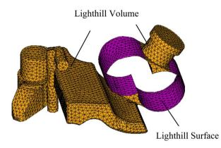
Figure 3. The grid of the acoustic source: Lighthill volume and Lighthill surface.
