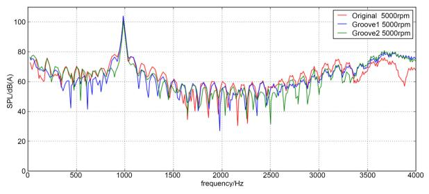
**Figure 8.** Sound pressure spectra: simulation results of original pump, unloading groove pump and unloading groove and diversion groove pump at 5000 rpm.
