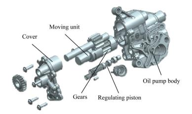
Figure 1. An exploded view of a variable displacement external gear pump.
