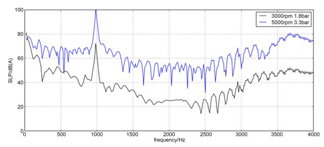
Figure 4. Simulated results of the A-weighted sound pressure levels at 3000 rpm (1.8 bar) and 5000 rpm (3.3 bar).
