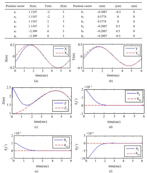
Figure 4. Plots of desired and actual position and orientation of the platform, (a)-(c) position in X-Y-Z directions, respectively, (d)-(f) orientation around X-Y-Z direction, respectively.
