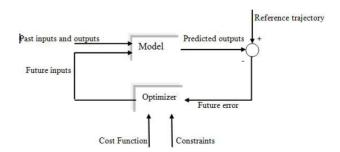
Figure 2. Basic structure of MPC.
