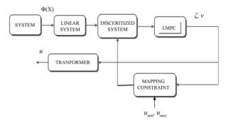
Figure 3. Schematic of control structure.
