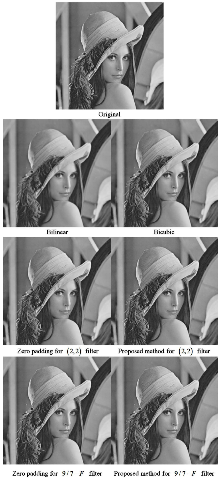
Figure 10. Image Lena reconstructed by bilinear, bicubic, zero padding and the proposed algorithm.
