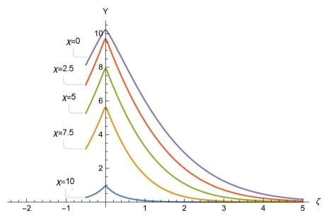
**Figure 7.** Plot of the diffusion momentum  $\Upsilon$  near the plate when it is streamlined by a viscous fluid. The dimensionless length of the plate is 10 and it is located on the axis of abscissa  $\chi$  at the interval (0,10). The values of the coordinate  $\chi$  are indicated on the left of the corresponding plot. The lower plot gives the values of the momentum at the beginning of the plate, the upper one at the end.
