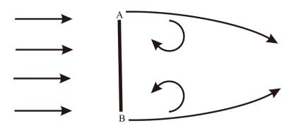
**Figure 3.** Shown is a thin plate located perpendicular to the running flow. The thickness of its slides at points A and B is much less than the diameter of the vortices occurring behind the plate.
