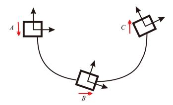
**Figure 2.** Nonpotential flow. The material particles turn changing their orientation in the flow at points *A*, *B*, *C*. The red arrows show the direction of the motion of the particles.
