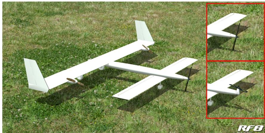
**Figure 6.** A canard airplane incorporating the roto-canard concept. The roto-canard was mounted on the nose section which was rotatable about the pitch axis (inset).
