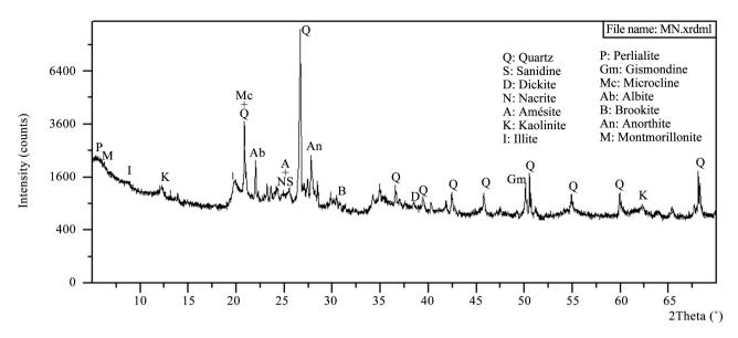
Figure 3. X-ray diffractogram of MN material.
