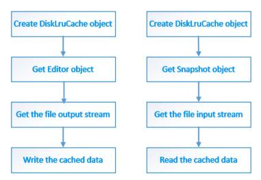
Figure 4. Write and read the disk cache data.
