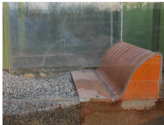
Figure 3. (a) Profile of fixed weir; (b) Installed weir model in channel.
