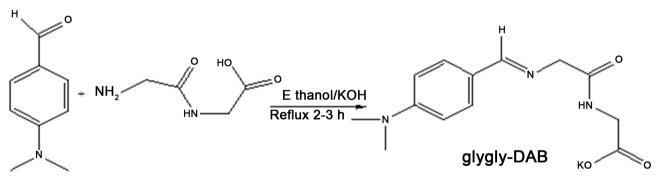
Figure 1. Equation for the synthesis of glygly-DAB.
