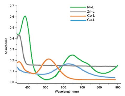
Figure 4. UV-vis spectra of glygly-DAB metal complexes.
