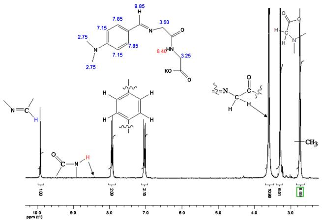
Figure 2. The <sup>1</sup>H-NMR spectrum and proposed structure of glygly-DAB ligand (L).
