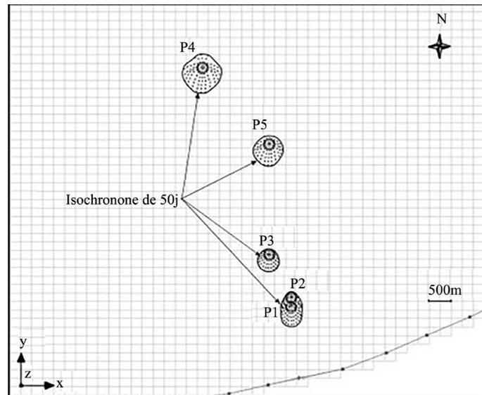
**Figure 7.** The closed protective perimeters of supply wells: 1951/27 (P1), 1950/27 (P2), 3061/27 (P3), 2024/27 (P4) and 1199/27 (P5).
