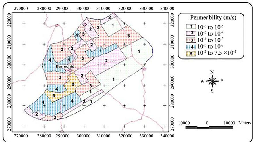
Figure 4. Distribution of the permeabilities resulting from steady-state calibration.
