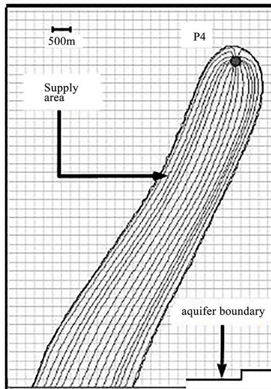
**Figure 10.** Enlarged view the feeding area of the borehole 1199/27 (P4).
