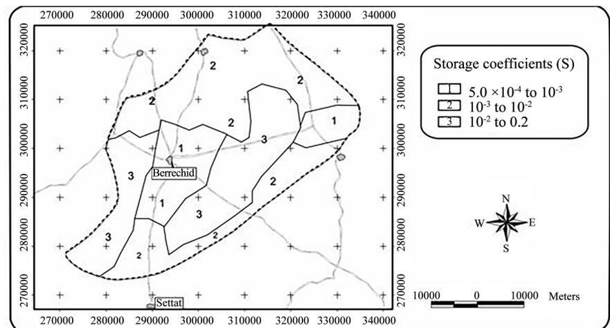
Figure 5. Distribution of storage coefficients from transient calibration.
