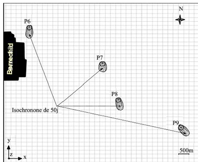
**Figure 8.** The closed protective perimeters of supply wells: 876/28 (P6), 3011/28 (P7), 1431/28 (P8) and 2149/28 (P9).
