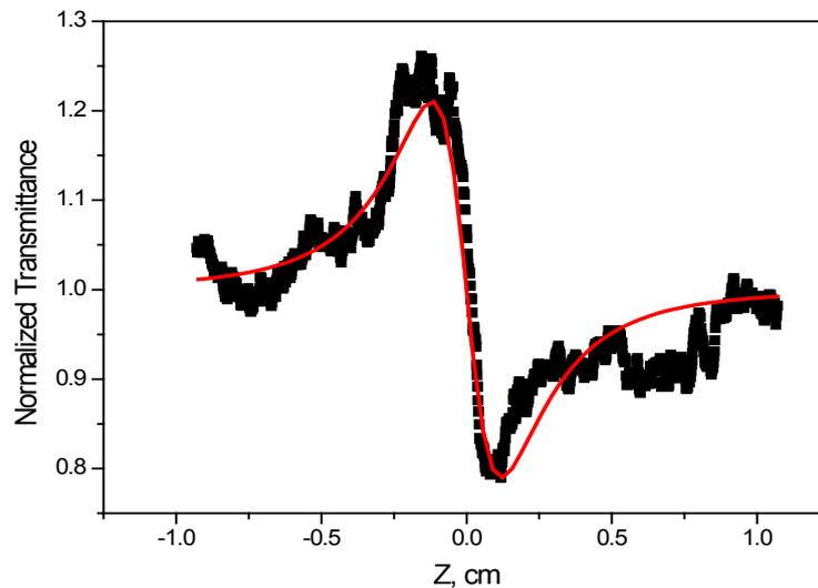
**Figure 5.** Closed aperture z-scan for Ag nanoparticles of size 25 nm at 514.5 nm and a line is a fit of equation 4 to experimental data.
