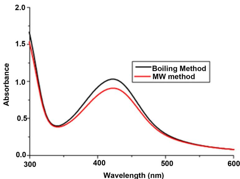
**Figure 1.** Absorption spectra of synthesized Ag NPs in water with different heating techniques.
