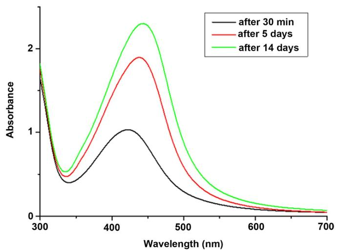
**Figure 3.** Variation of the SPR absorption peak with respect to the time for Ag nanoparticles prepared by boiling method.
