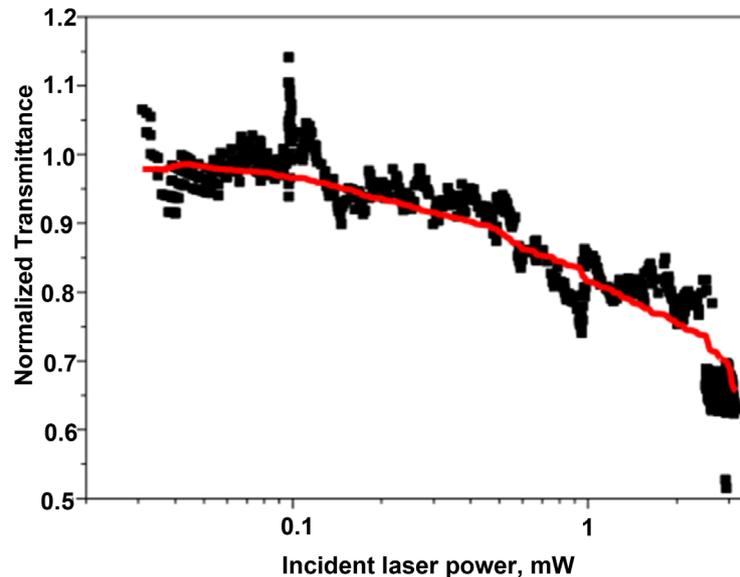
**Figure 7.** The optical limiting behaviour of Ag nanoparticle of size 25 nm at an excitation wavelength of 514.5 nm.
