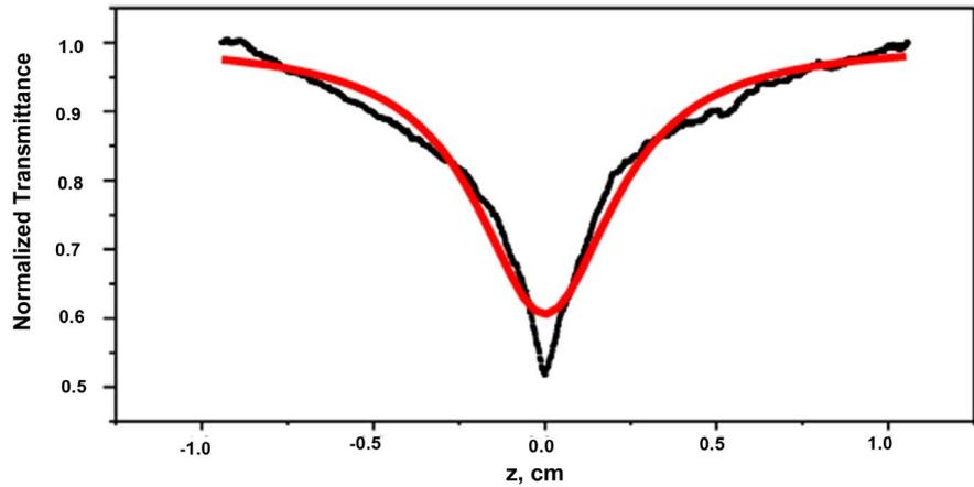
**Figure 4.** Open aperture Z-scan signal of Ag nanoparticles of diameter 15 nm at 488 nm and a line is a fit of equation 1 to experimental data.
