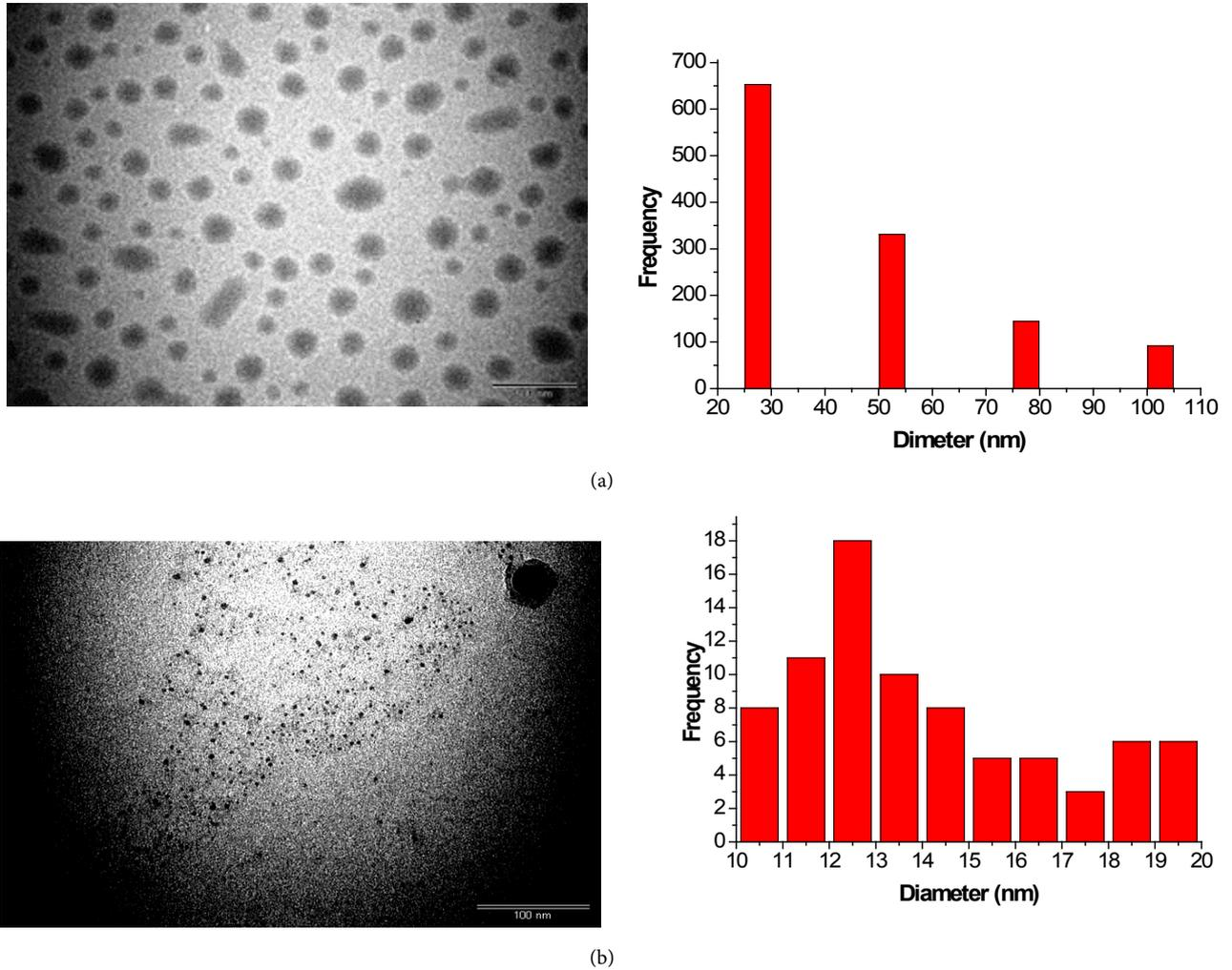
**Figure 2.** Transmission Electron Microscopy image and corresponding particle size distribution using J-image software (a) boiling method. (b) Microwave method.
