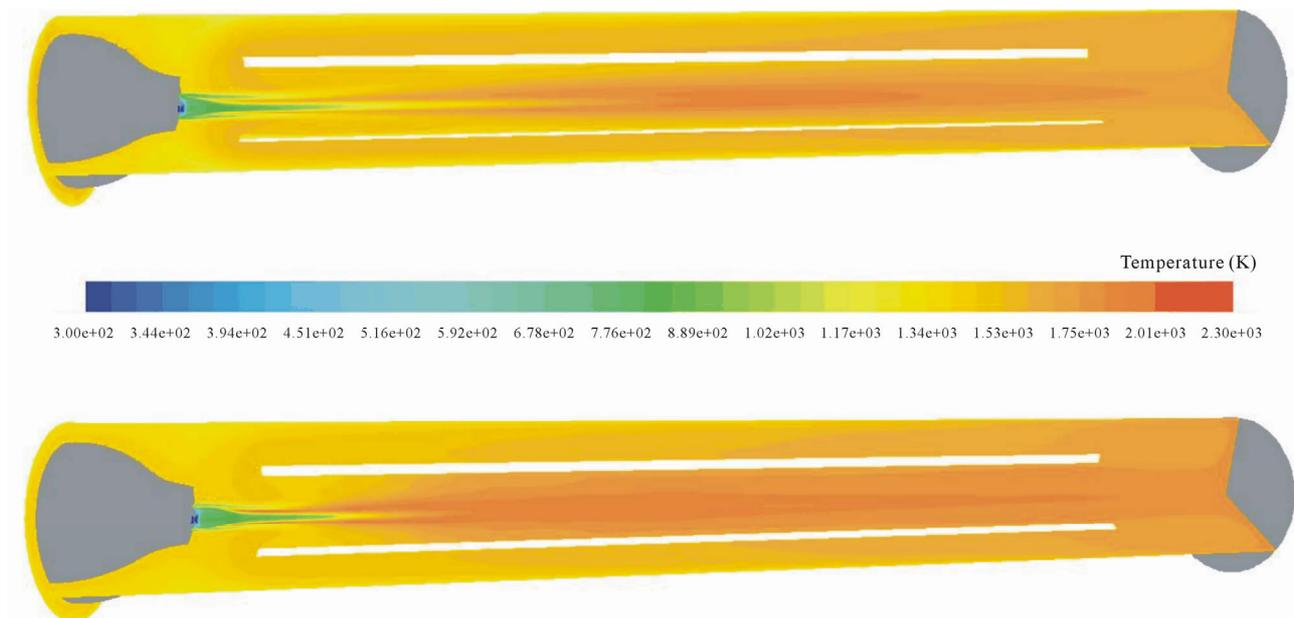
Figure 5. Top: RANS field of temperature. Bottom: averaged LES.
