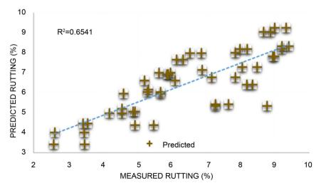
Figure 6. Predicted rutting vs Measured rutting.
