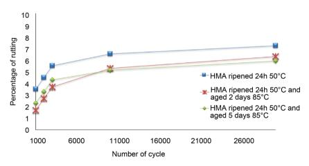
Figure 3. Impact of aging on HMA in terms of resistance to rutting.
