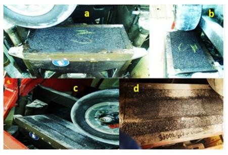
**Figure 2.** Rutted slabs of HMA rehabilitated with Micro-surfacing before and after rutting test (30,000 cycles) (a) Plate of HMA before rutting; (b) Plate of HMA before rutting; (c) Plate of HMA after 10,000 rutting cycles; (d) Plate of HMA after 30,000 rutting cycles.
