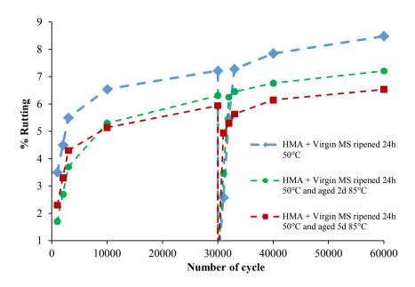
**Figure 4.** Impact of aging on HMA/ virgin micro-surfacing in terms of resistance to rutting.
