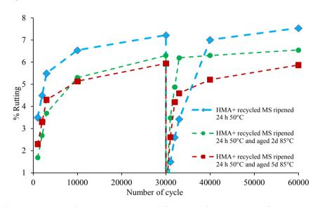
Figure 5. Impact of aging on HMA/ recycled micro-surfacing in terms of resistance to rutting.
