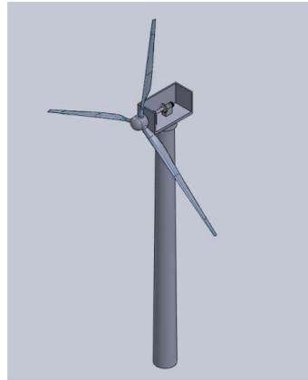
**Figure 4.** Entire HAWT geometry.
