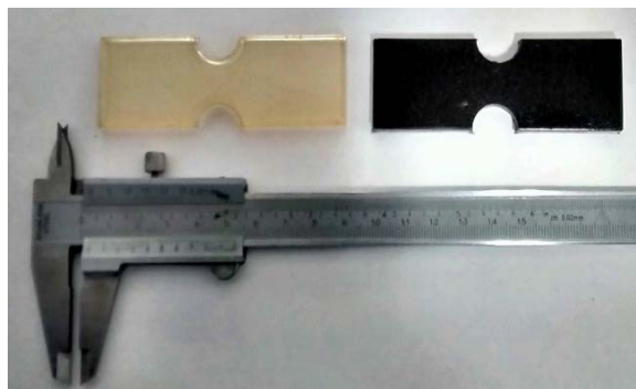
Figure 2. Photograph showing the shape and size of the tensile elastomeric PU composite samples fabricated without (white) and with 10 wt% GO-MG (black).
