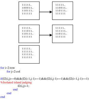
Figure 3. Example of pseudo vessel removal.
