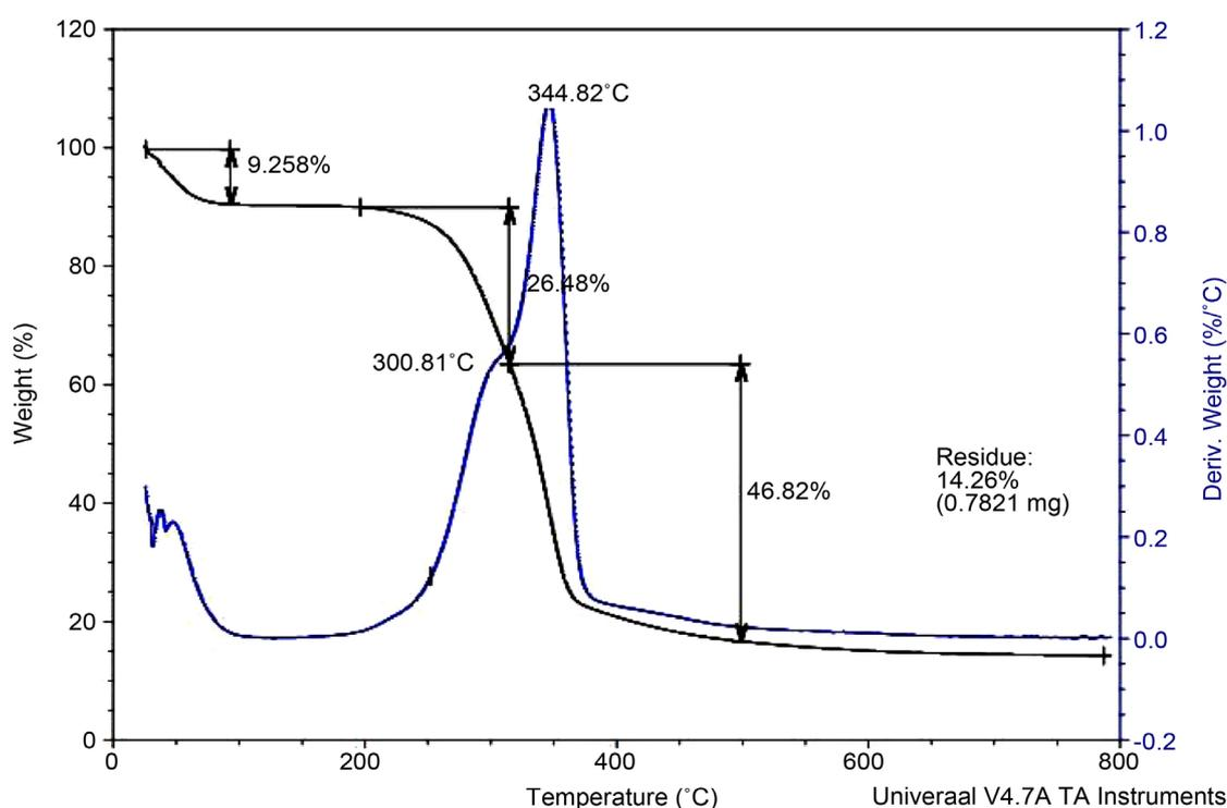
**Figure 1.** Thermogravimetric curve of sugarcane bagasse produced in Rio Grande do Sul.
