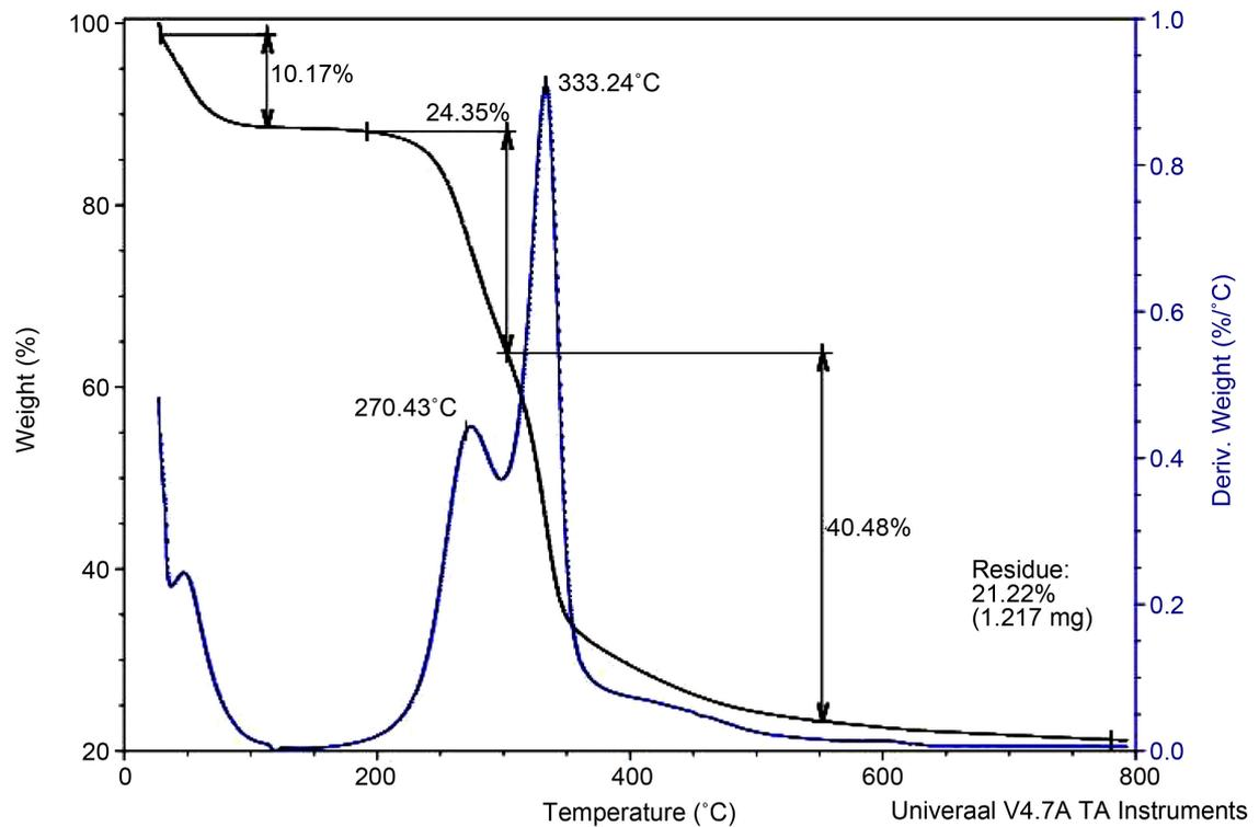
**Figure 2.** Thermogravimetric curve of sugarcane straw produced in Rio Grande do Sul.
