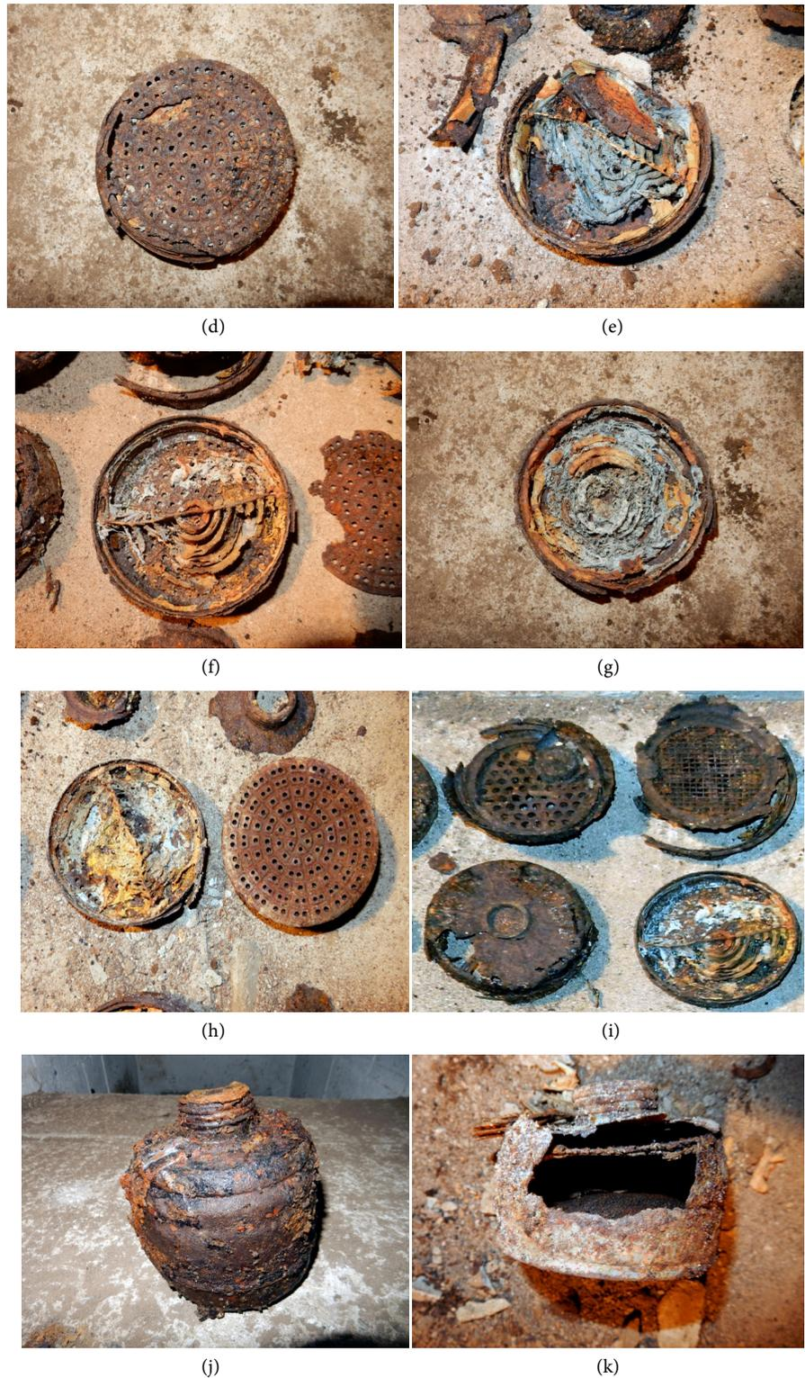
**Figure 7.** *L 479* discovered components of gas mask filtering cartridges (a) Overview; (b) Covers and pots of unknown filtering cartridges; (c) Upper line: *FE 39* cover and unknown type cover, lower line: *FE 42* covers; (d) *FE 37* cover; (e) Unknown cover; (f) Unknown cover; (g) Unknown cover; (h) Unknown cover and *FE 37* cover; (i) Upper line: unknown covers, lower line: *FE 41* cover and unknown cover; (j) Complete *FE 37* filtering cartridge; (k) Complete *FE 41* filtering cartridges.
