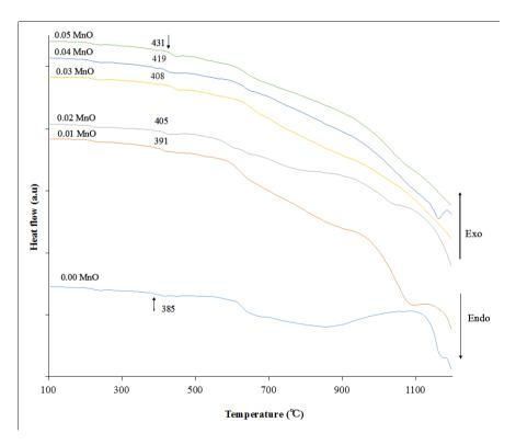
Figure 2. DSC curve for heat-treated glass sample.
