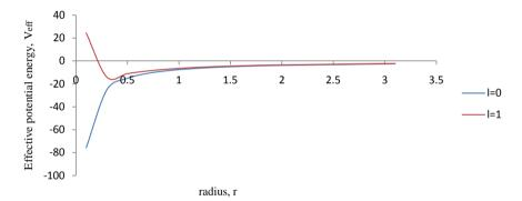
**Figure 6.** More general exponential screened coulomb plus Yukawa (MGESCY) potential versus r with  $V_0 = 2.75 \, \text{MeV}$ ,  $V_0 = 2.75 \, \text{MeV}$  and  $\alpha = 0.01$  for l = 0 and l = 1.
