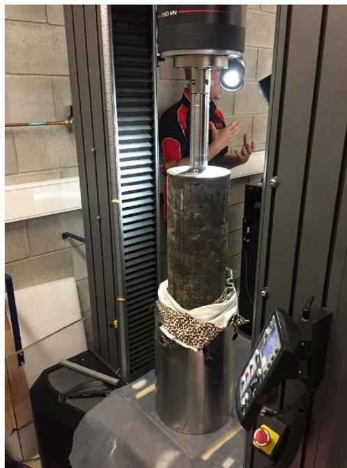
**Figure 1.** Bentonite plug under test using an Instron 250 kN electro-mechanical loading frame. A split collar was designed to sit against the top face of the cylinder loading seat to guarantee axial alignment of the casing with the test machine.
