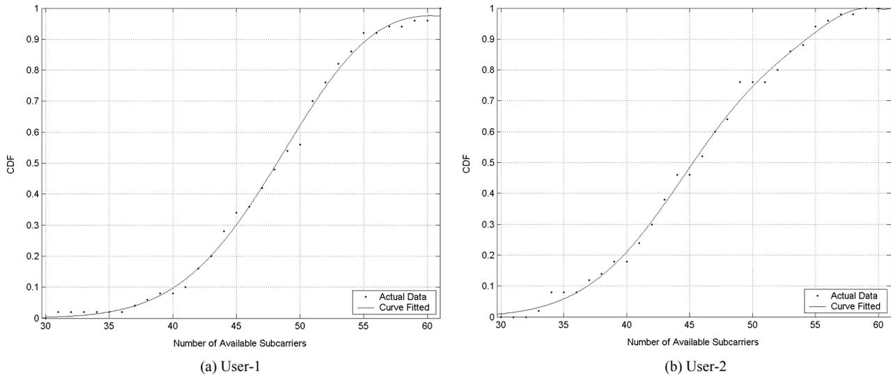
**Figure 6. Cumulative distribution function of the available subcarriers.**
