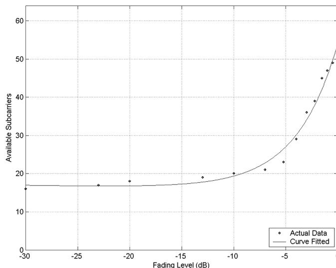
Figure 9. Number of available subcarriers versus fading level.
