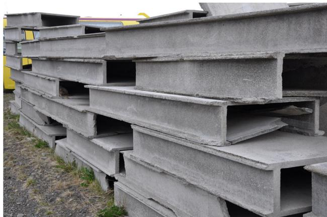
**Figure 5.** Faulty CBPB box elements stacked outdoors.
