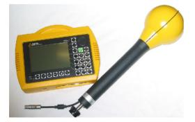
Figure 2. Narda narrowband field meter (SRM3000).
