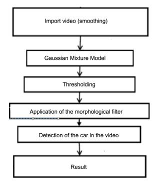
Figure 1. Diagram of the proposed method.
