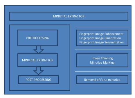
Figure 3. Simplified fingerprint system.
