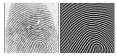
Figure 5. Histogram equalization with image enhancement.
