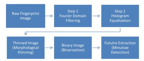
Figure 2. Block diagram for fingerprint recognition.
