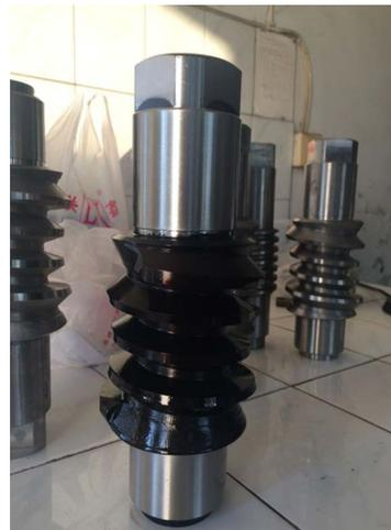
**Figure 12.** Worms with trivalent chromium hard chromium coatings.
