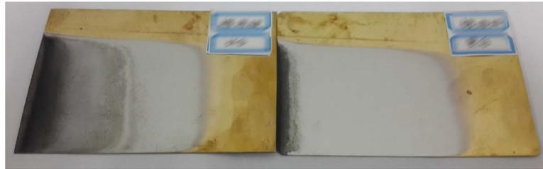
**Figure 1.** Hull specimen of trivalent chromium plating.
