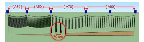
**Figure 2.** Layout of the production line with the different distances between the suspended mussel socks and their vicinity to the bottom.
