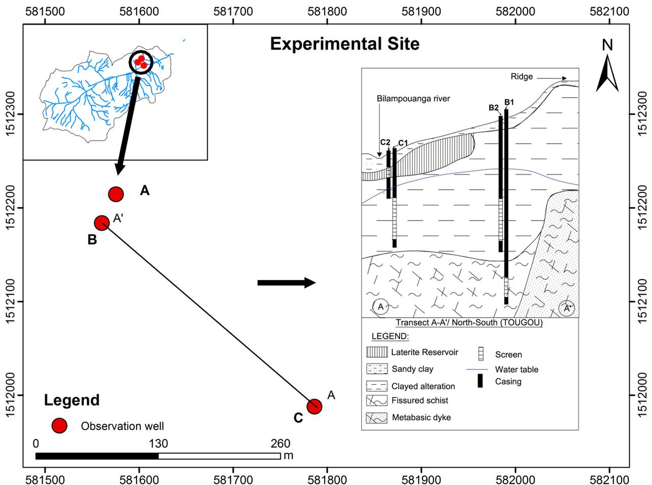
**Figure 3.** Location and design of piezometers cluster on Tougou experimental site (modified from IWACO [13]).
