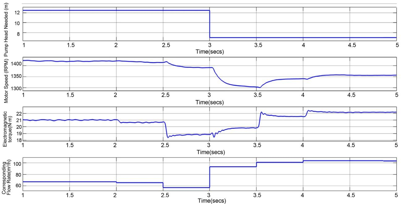
Figure 21. Simulation results of  $H$ ,  $N$ ,  $T_e$  and  $Q$ .
