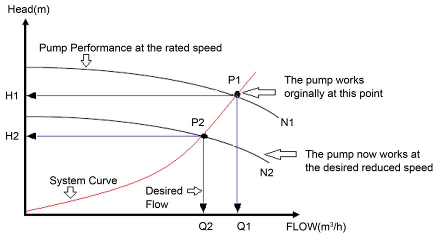
Figure 10. Variable speed pump performance curves.
