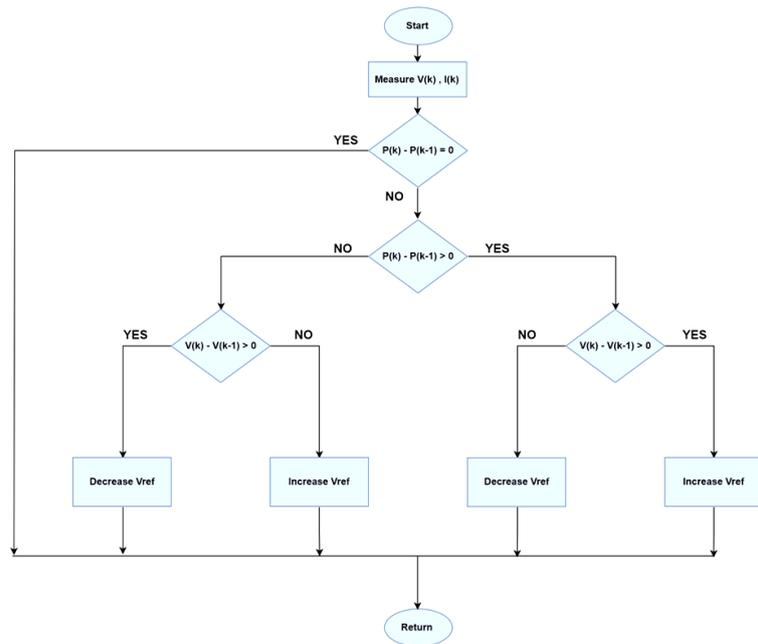
Figure 4. Flowchart of the perturb and observe algorithm.
