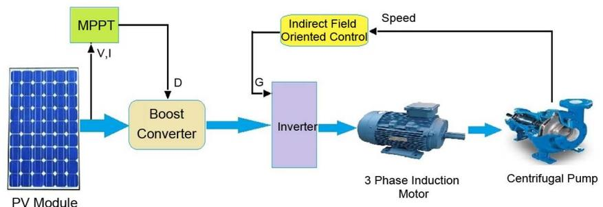
**Figure 1.** Proposed photovoltaic water pumping system.
