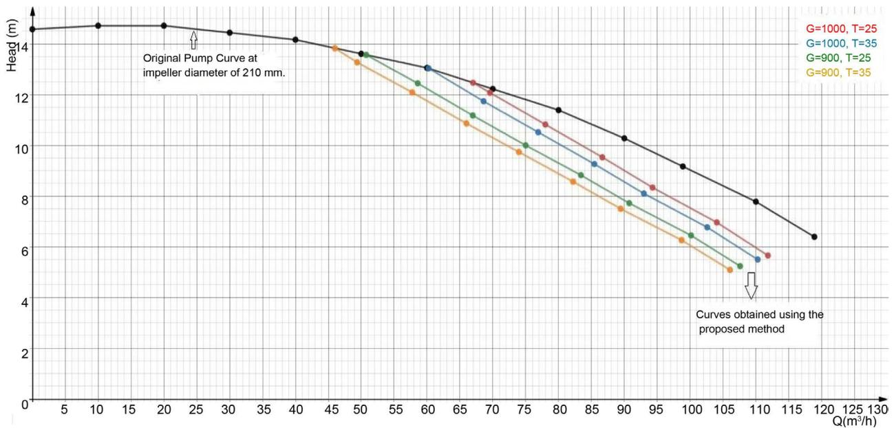
**Figure 15.** (Head Vs. Flow) curves obtained using the proposed method.
