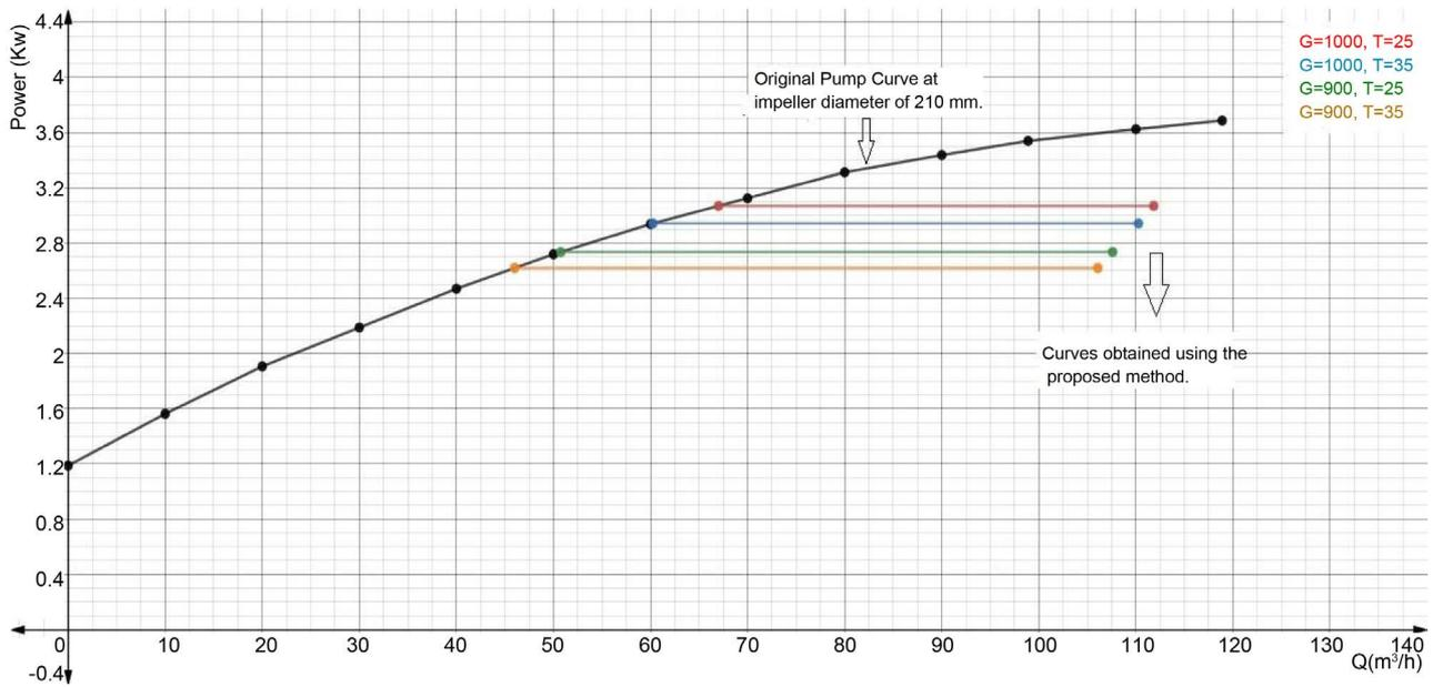
Figure 16. (Power vs. Flow) curves obtained using the proposed method.
