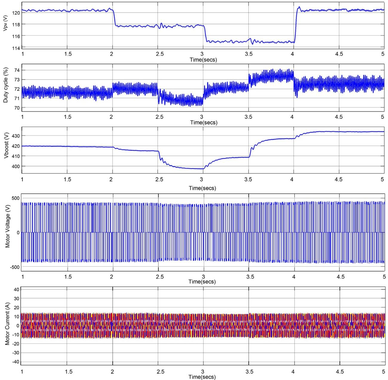
**Figure 19.** Simulation results of  $V_{pv}$ ,  $D$ ,  $V_{boost}$ ,  $V_{inverter}$  and  $I_m$ .
