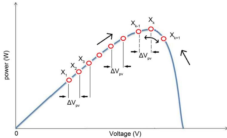
Figure 3. Operation of perturb and observe algorithm.
