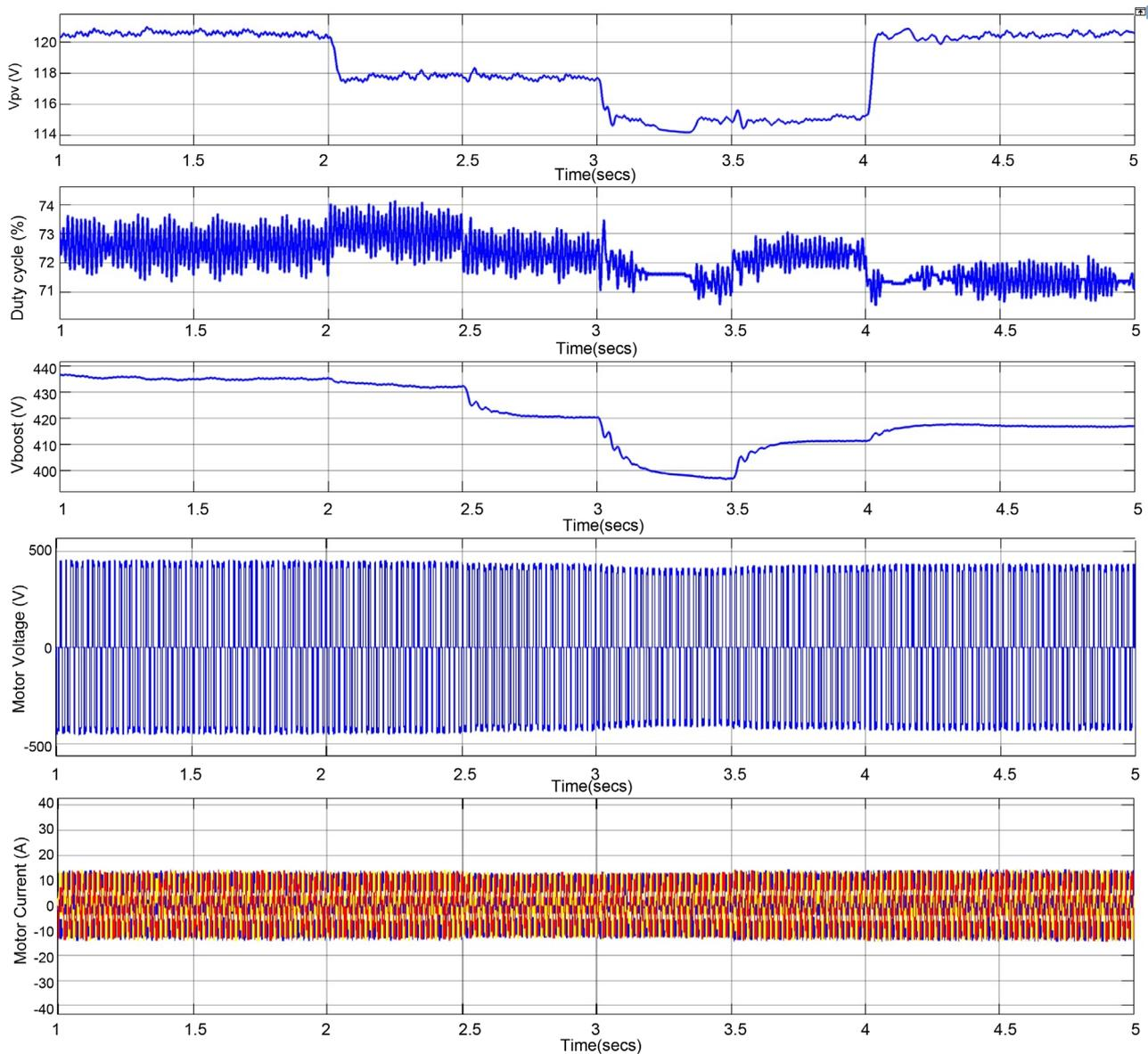
**Figure 22.** Simulation results of  $V_{pv}$ ,  $D$ ,  $V_{boost}$ ,  $V_{inverter}$  and  $I_m$ .
