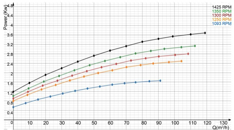
Figure 12. (Power vs. Flow) pump performance curves (variable speed, fixed impeller diameter of 210 mm).
