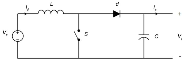
**Figure 5.** Step-Up (Boost) converter configuration.
