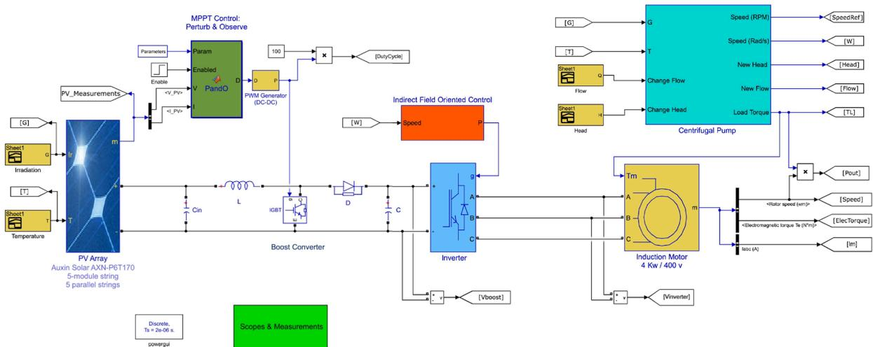
**Figure 13.** Matlab/Simulink model of PV water Pump.
