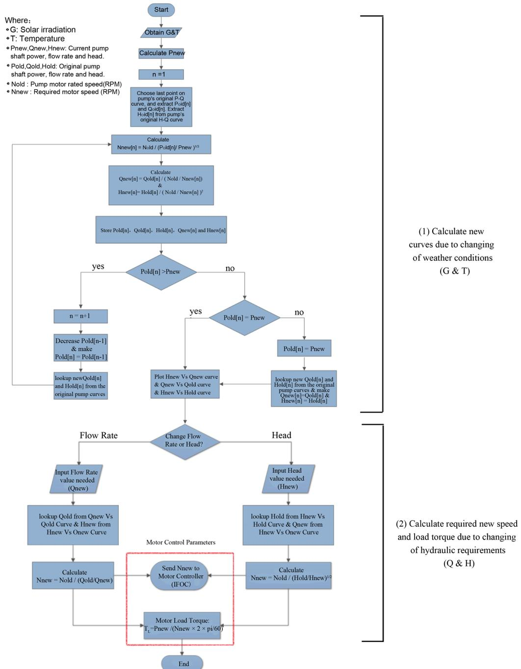
**Figure 14.** Proposed method for controlling the pump performance using the Affinity laws.
