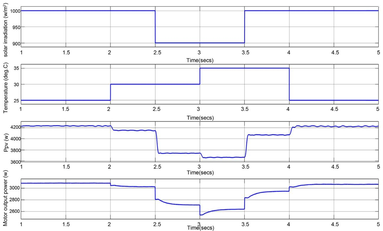
Figure 17. Simulation results of  $G$ ,  $T$ ,  $P_{pv}$  and  $P_{out}$ .
