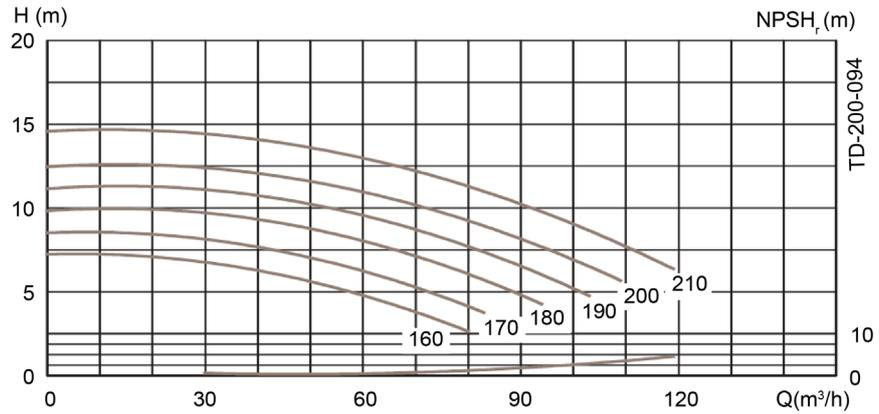
**Figure 8.** (Head vs. Flow) pump performance curves (variable impeller diameter, constant speed of 1425 RPM).
