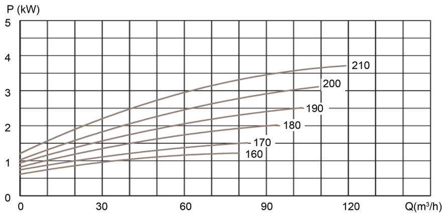
**Figure 9.** (Power vs. Flow) pump performance curves (variable impeller diameter, constant speed of 1425 RPM).
