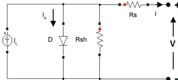
**Figure 2.** Equivalent circuit of a PV cell.
