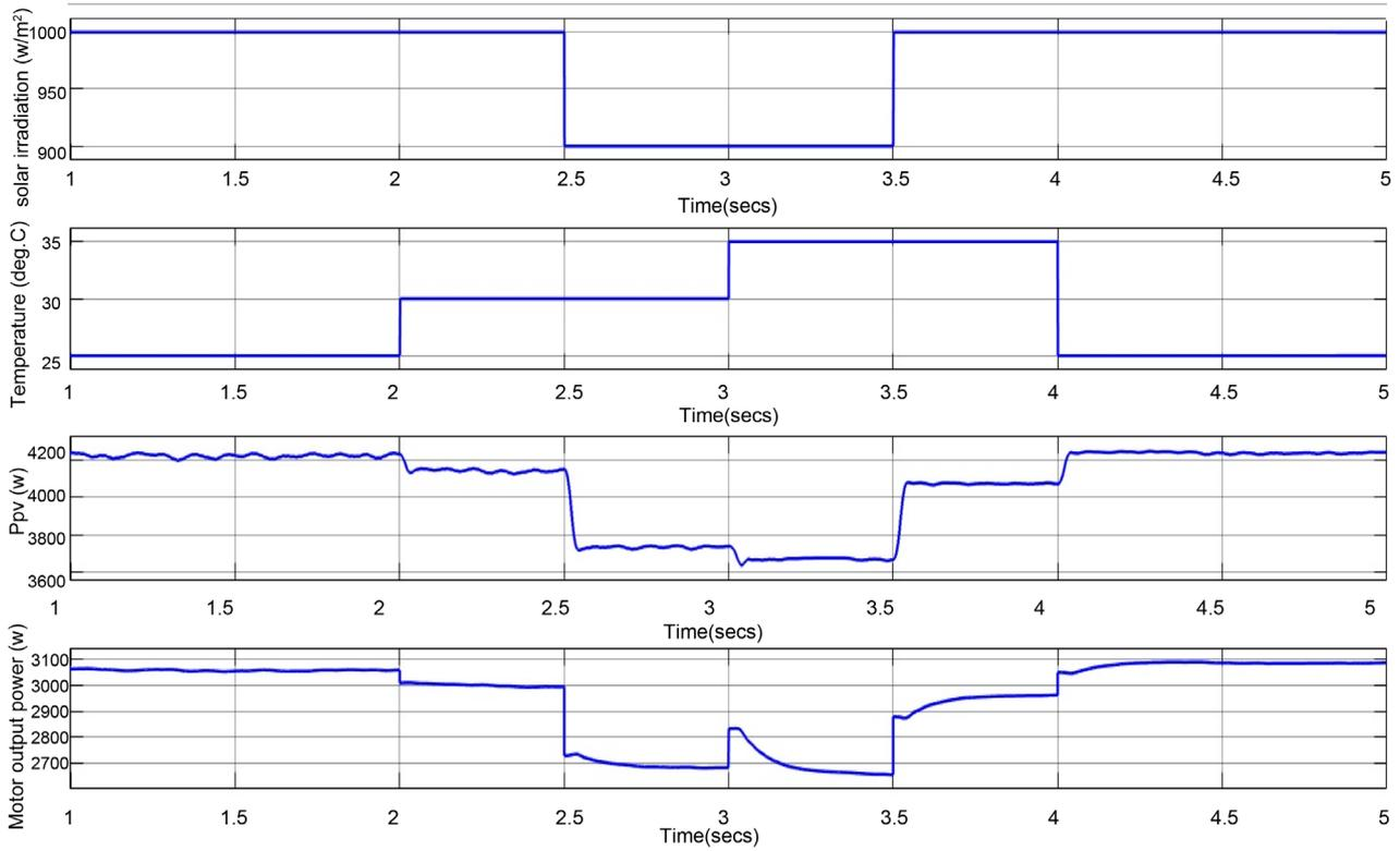
Figure 20. Simulation results of  $G$ ,  $T$ ,  $P_{pv}$  and  $P_{out}$ .
