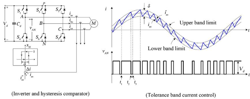
**Figure 7.** Current controlled voltage source inverter.
