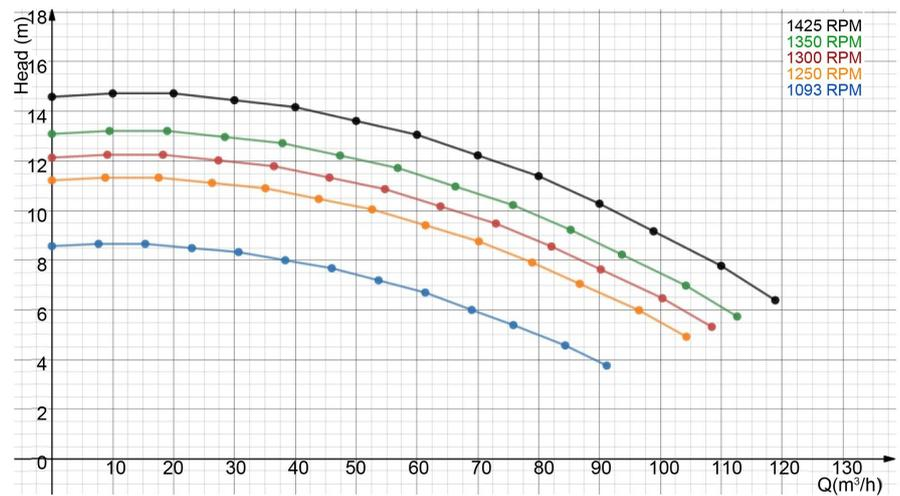
Figure 11. (Head vs. Flow) pump performance curves (variable speed, fixed impeller diameter of 210 mm).
