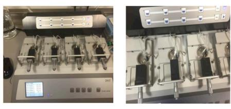
Figure 1. Multiwire myograph system (DMT 620M).
