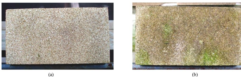
**Figure 4.** (a) shows a relatively unsoiled Blaxter Sandstone sample exposed in Belfast (August 2009–December 2010), (b) shows a Blaxter Sandstone sample exposed in the wet west of NI, Omagh over the same period. Both samples were north facing.
