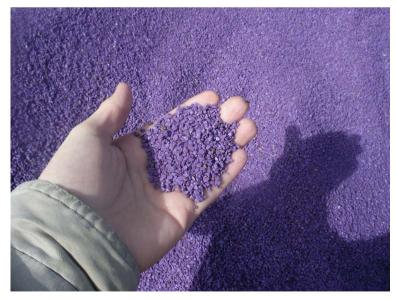
Figure 4. Close up of colored pavement tire-grip material.
