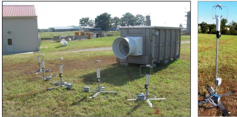
Figure 3. The 3D ultrasonic anemometer assemblies (left: anemometer on the post with data logger and battery power supply) and illustration of the adjustable heights of the anemometer assembly on the post (right).
