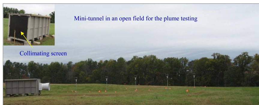
Figure 2. The wooden mini-tunnel with a 0.6 m (24-in) axial ventilation fan on the one end and the collimating screen on the other end.
