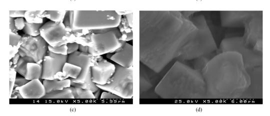
Figure 3. SEM micrographs of fractured surface of  $(1 - x)K_{0.5}Na_{0.5}NbO_{3-x}LiSbO_3$  pellets (x = 0.045) sintered at (a) 1060°C; (b) 1080°C, (c) 1100°C and (d) 1120°C.
