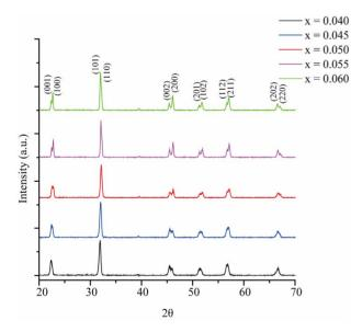
Figure 1. Room temperature XRD pattern of  $(1 - x)K_{0.5}$ Na<sub>0.5</sub>NbO<sub>3-x</sub>LiSbO<sub>3</sub> ceramics.
