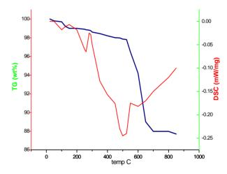
Figure 5. DSC and TGA curves of  $(1 - x)K_{0.5}Na_{0.5}NbO_{3-x}$ LiSbO<sub>3</sub> with x = 0.045.
