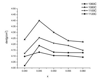
Figure 4. Density of  $(1 - x)K_{0.5}Na_{0.5}NbO_{3-x}LiSbO_3$  ceramics as a function of x.
