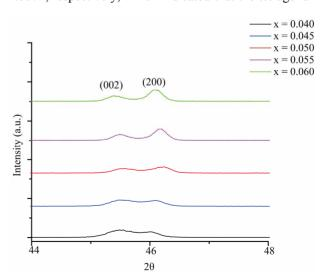
Figure 2. XRD patterns of the ceramics in the ranges of  $2\theta$  from 44° to 48° of  $(1 - x)K_{0.5}Na_{0.5}NbO_{3-x}LiSbO_3$  ceramics.
