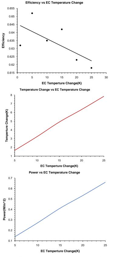
**Figure 6.** Efficiency, temperature change and power change as a function of temperature change of EC materials.
