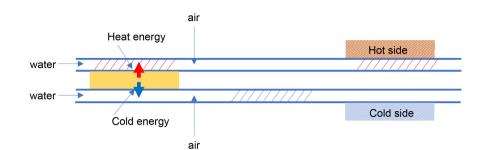
Figure 2. Design of electrocaloric cooling system.
