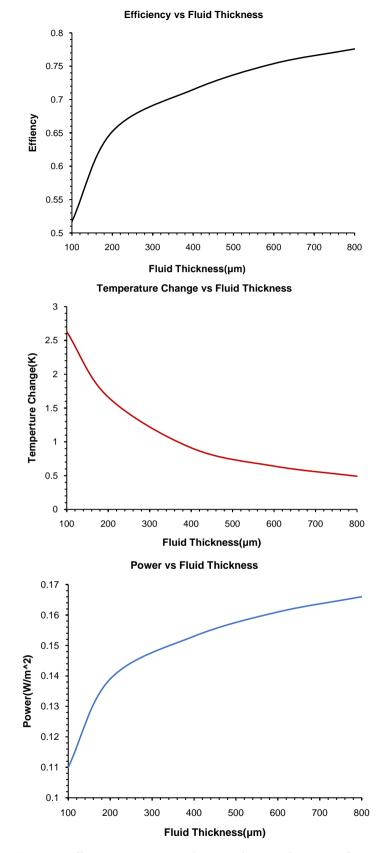
**Figure 4**. Efficiency, temperature change and power change as a function of fluid thickness.
