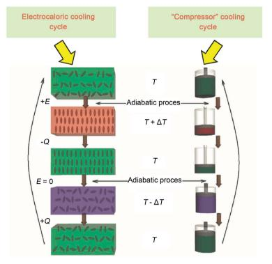
Figure 1. Comparison of Electrocaloric cooling cycle and "Compressor" cooling cycle.
