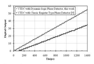
Figure 16. Comparison of the digital output characteristics of the single-stage VTDC with the dynamic-logic phase detector with the characteristics of the single-stage VTDC with the classic register-type phase detector from [6].
