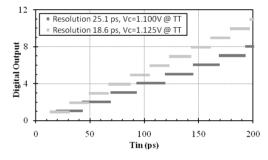
Figure 17. Digital output characteristics of the single-stage VTDC with the dynamic-logic phase detector in which the control voltage has been used to set up different time measurement resolution. Only the 0 - 200 ps fraction of the entire time scale has been shown for simplicity. (A small vertical offset in the digital output has been introduced for better readability).
