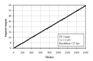
Figure 15. Digital output characteristic of the single-stage VTDC with the dynamic-logic phase detector (TT corner).
