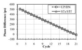
Figure 10. Zero dead-zone characteristic of the Delayed-Input-Pulse Phase Frequency Detector.
