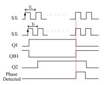
Figure 3. Timing diagram of the correct phase detection [4].
