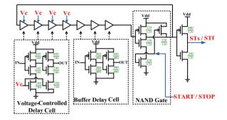
Figure 6. Schematic of the triggerable voltage-controlled oscillator.
