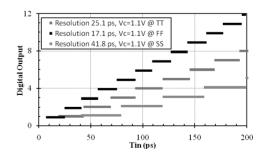
Figure 18. Variability of the digital output characteristics of the single-stage VTDC with the dynamic-logic phase detector as a function of process variations (in the TT, FF, and SS process corners), for a constant control voltage,  $V_c = 1.10$  V. Only the 0 - 200 ps fraction of the time scale has been shown for simplicity. (A small vertical offset in the digital output has been introduced for better readability).
