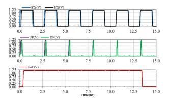
Figure 12. Timing diagram of dynamic-logic phase detector.
