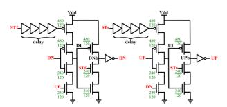
Figure 9. Delay-input-pulse phase frequency detector [11].
