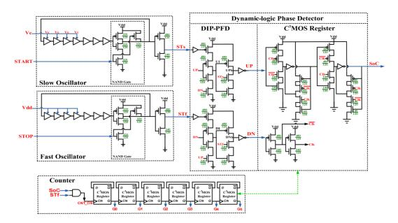
Figure 14. Schematic diagram of the single-stage VTDC.
