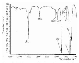
Figure 3. FT-IR spectra of linoleic acid protected silver nanoparticles dispersed in chloroform.
