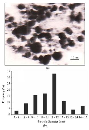
Figure 2. (a) TEM image of silver nanoparticles; (b) particle size distribution.
