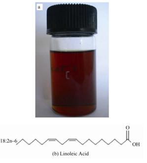
Figure 1. (a) Silver nanoparticles dispersed in chloroform showing reddish brown colour; (b) chemical structure of linoleic acid.
