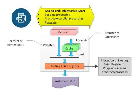
Figure 2. End-to-end prefetching implementation architecture.
