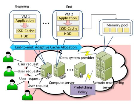
Figure 1. Adaptive cache allocation in the end-to-end cloud environment.
