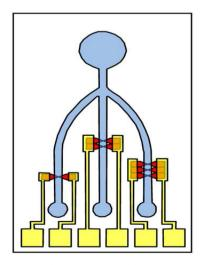
Figure 2. A lab-on-a-chip microfluidic device showing the inlet and outlets. (Source: Sharma et al., 2013 [15]).
