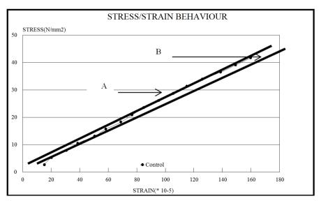
Control-100% Medium Sand; A-10% Sand replaced with limestone dust; B-20% Sand replaced with limestone dust.
