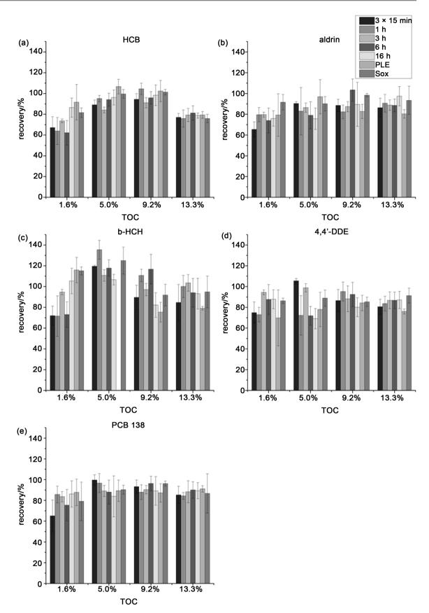
**Figure 1.** Recovery of the analytes (a) HCB, (b) aldrin, (c)  $\beta$ -HCH, d) 4,4'-DDE, and (e) PCB 138 in % of spiked concentration. The error bars indicate the standard deviation (n = 4).
