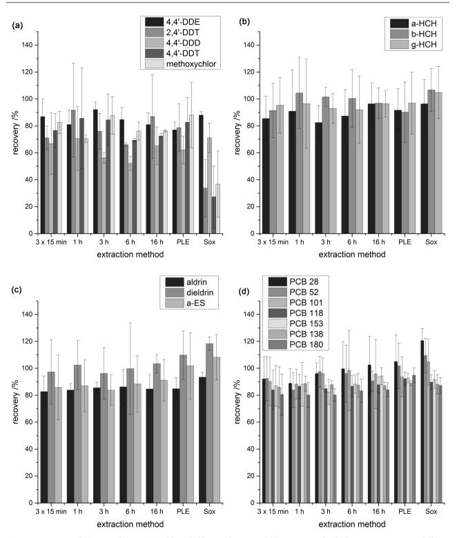
**Figure 3.** Recovery of (a) DDX, (b) HCH, (c) aldrin, dieldrin, and  $\alpha$ -ES, and (d) PCB in % of spiked concentration using different extraction techniques. The error bars indicate the standard deviation (n = 4).
