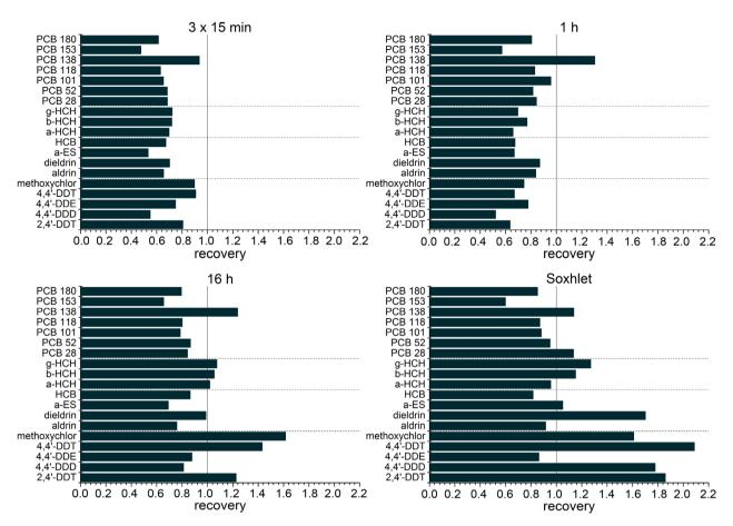
**Figure 2.** Recoveries as assessed for the measurands under consideration in the low-level TOC soil using SLE with  $3 \times 15$  min, 1 h, 16 h and Soxhlet extraction. All "explainable" values are below the unity line (recovery = 1), all unexpected above.
