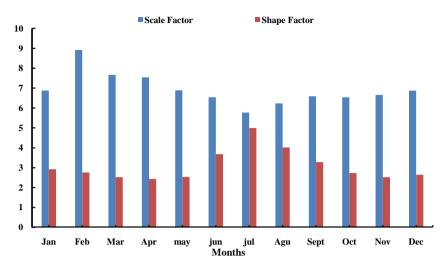
Figure 5. Monthly Weibull distribution parameters at 50 meters.
