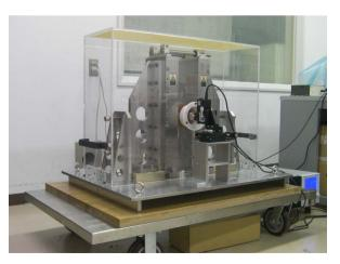
**Figure 1.** A photograph of our second-generation scanner for magnetic particle imaging (MPI).
